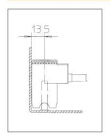
MINIMUM DISTANCE FROM STUD CENTRE TO INSIDE FACE OF VERTICAL WALL IS 13.5mm
