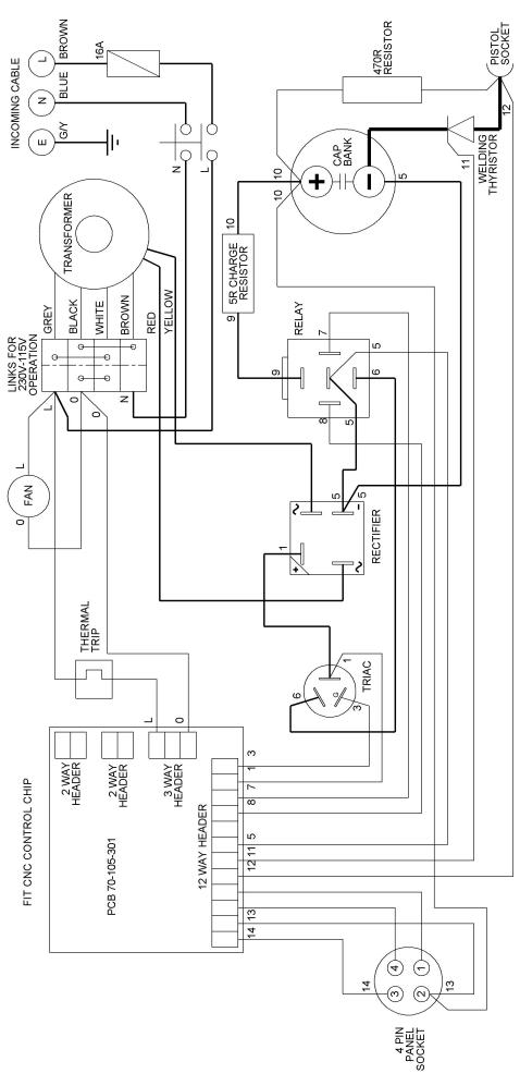
CNC CONTACT CONTROLLER. MODELS M8, M9 & M10 **WIRING SCHEMATIC**
