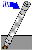
A simpler test may be achieved by bending the stud over 30° using a hide mallet.
