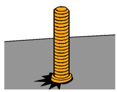
A one sided stud weld (arc blow) is usually caused by incorrect earthing of the work piece. This may be corrected by placing the welding earths opposite each other across the area where the weld is to occur.
