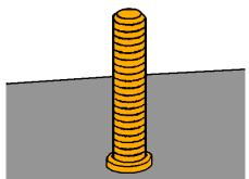
A cold stud weld is noticeable by undercutting of the flange and lack of / minimal formation of spatter. A cold weld is usually caused by too little energy and / or too high spring pressure.
