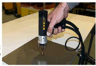
Visually inspect the weld. A good weld will result in an all round weld with a small visible witness of spatter surrounding the flange of the stud.
