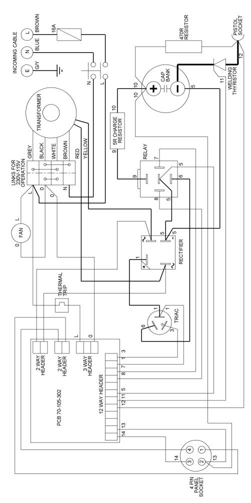
LIFT GAP CONTROLLER. MODELS M8, M9 & M10 **WIRING SCHEMATIC**
