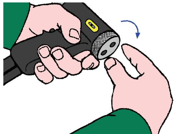
**Switch the controller ON.**
