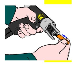
Tighten the chuck locking nut with the box spanner provided. A gentle pressure is all that is required. Over tightening may result in damage to your pistol.
