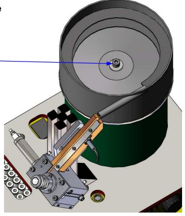
Align the output tube of the bowl with the track of the escapement and ——re-tighten the central screw.
