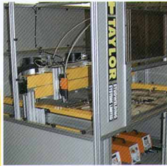
CNC system welding 2 components simultaneously
