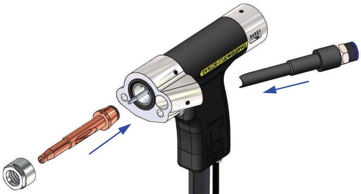
Select the correct size feed hose for the stud to be used (see page 36) and push into the feed hose gland.
