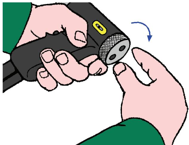
**To prevent inadvertent movement of the lift adjustment, the end cap can be locked into place by tightening the grub screw in the end cap.**
